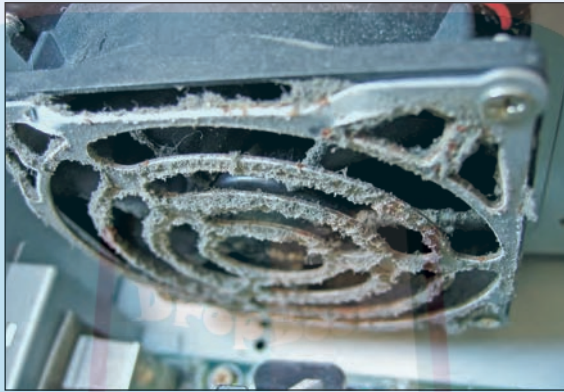
Color Plate 33: Don't let dust collect inside your PC. And when blowing off the dust with compressed air, do it outdoors, so the dust doesn't fill your lungs and get all over the room.
